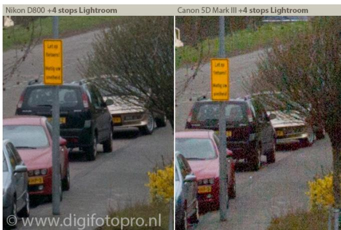
Figure 1: 5D3 vs D800 shadow recovery: ISO 100, f/8, 1/2000, +4EV in post.
